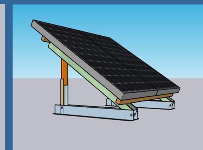
Figure 2. A view of the Design of Tilt angle adjustment Panel stand.
